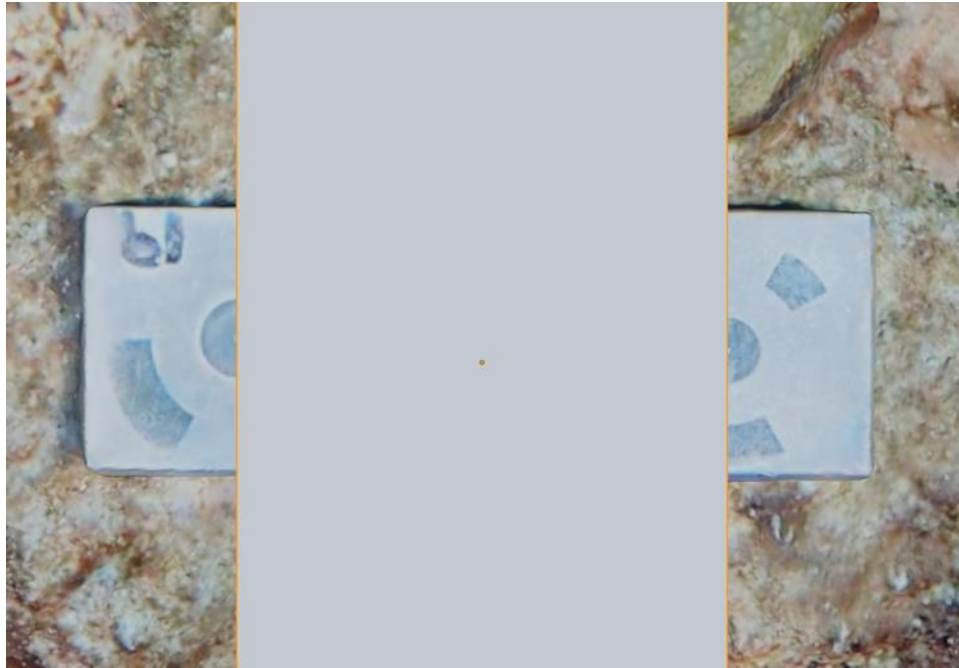
The width of the gray, artificial scale bar was set to 0.1m and now aligns with the known distance of 0.1m between the centers of the coded targets in the model's actual scale bar.
