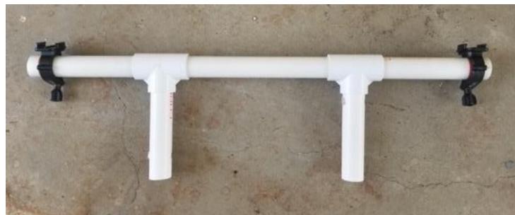
The dual-camera "hammerhead" rig, with two GoPro mounts attached (clamps are positioned so that cameras are approximately 60cm apart).
