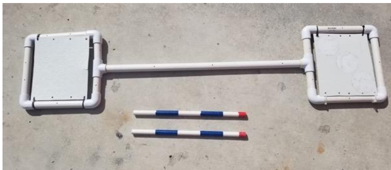
Old square-end (above) and stick (below) scale bars, all made from PVC. Agisoft coded targets may be printed separately and affixed to the square-end bar with waterproof stickers or glue.
